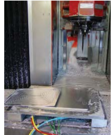
Sheet metal parts are clamped deformation-free by means of vacuum clamping plates
