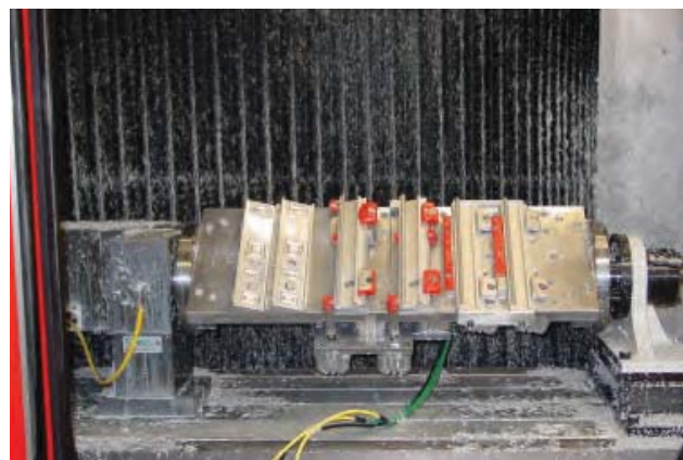
Swiveling device for multiple clamping of aluminium design rails
