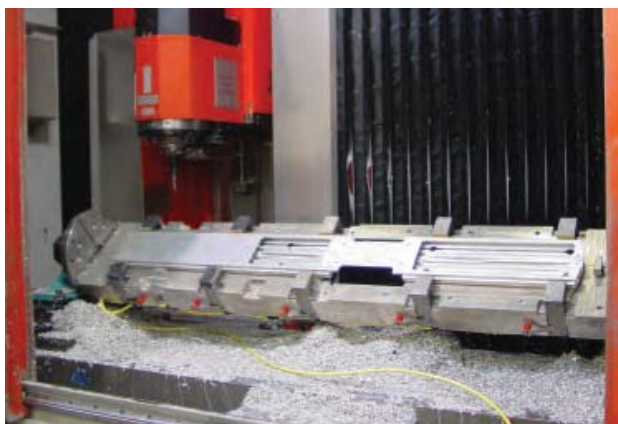
Swiveling device for clamping of extremely damageable hollow chambered rails
