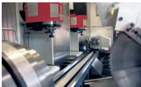
Working area with 2 traveling columns, counterspindle vs. CNC rotary table and saw unit
