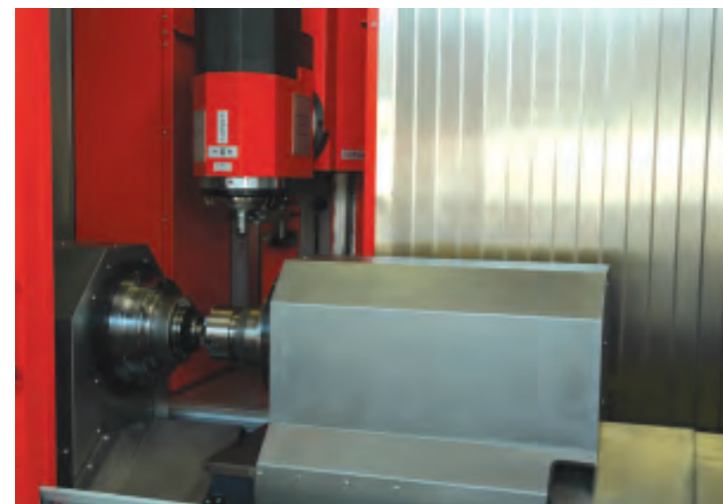
Work part transfer into the opposed spindle
