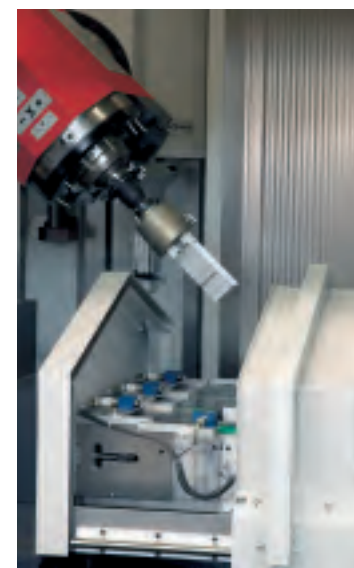
NC-gripper depositing a work part
