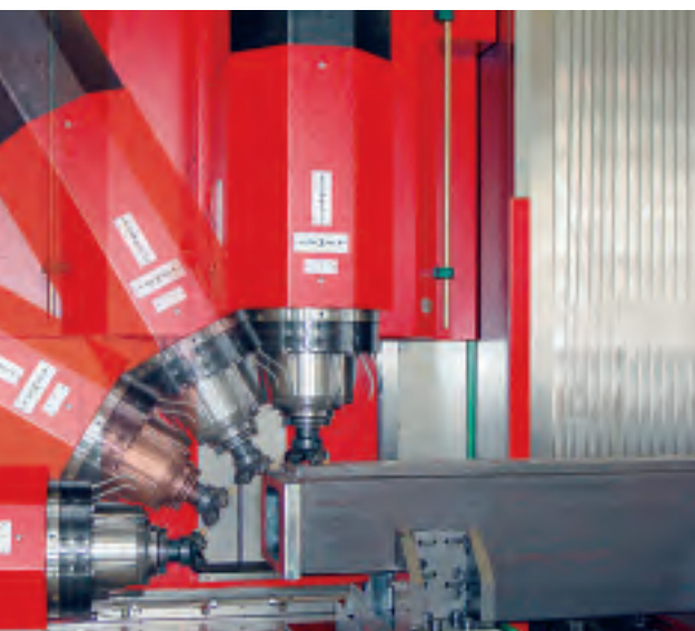
Swivel head +/- 105° continuously variable
