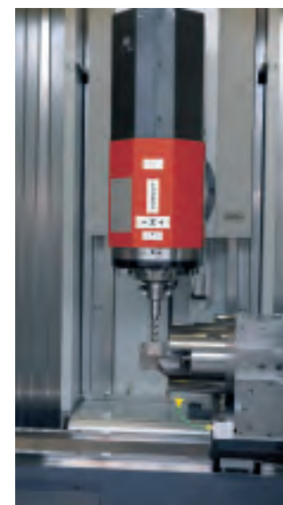
Machining at opposite spindle
