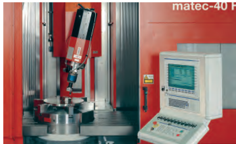
Integrated rotary table with direct drive, max. speed = 500 rpm
