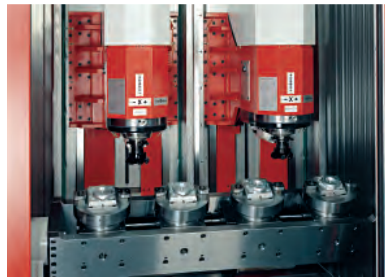
Right-sided working area with tilting table and clamping device
