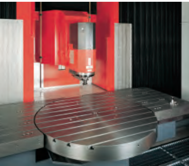
matec-30 HV with integrated rotary table 1450 mm
