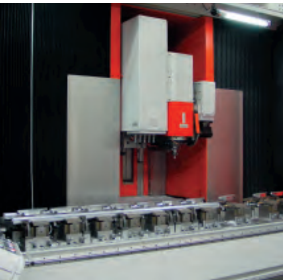
matec-30 L special clamping devices for aluminium profiles
