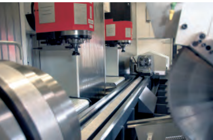
Working area with 2 traveling columns, opposed spindle vs. CNC rotary table and saw unit
