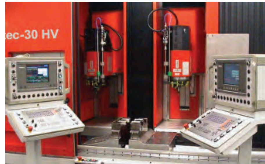
matec-30 HV with two traveling columns and 9 CNC axes
