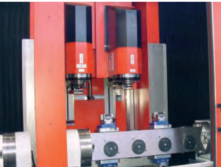
Double spindle with tilting table
