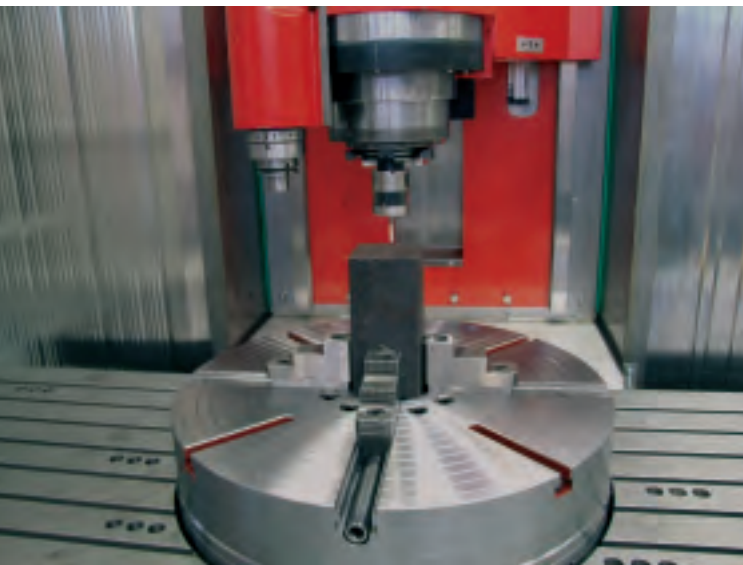
Working area with integrated rotary table and mounted jaw chuck
